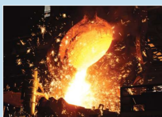
Liquid metal chemical correction in induction furnace
